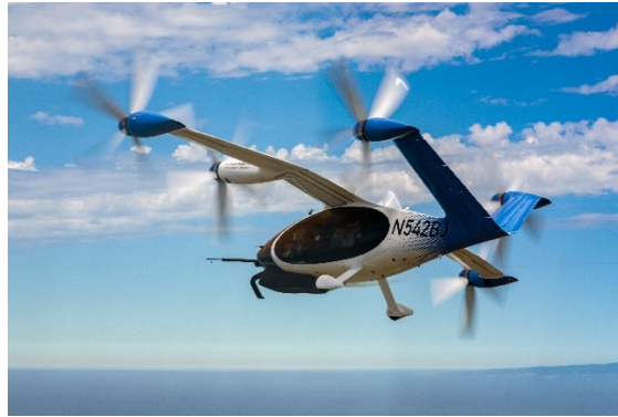
Figure 1: Joby's hydrogen-electric, vertical take-off and landing demonstrator aircraft completed a landmark 523 mile flight in July 2024. 14
