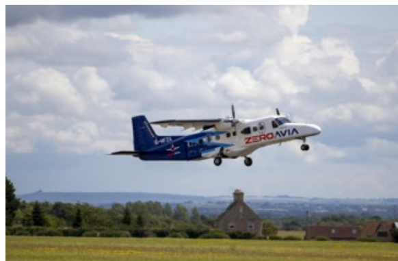
Figure 3: ZeroAvia Dornier 228 on takeoff during 10th flight test of prototype ZA600 hydrogen-electric engine. 16
